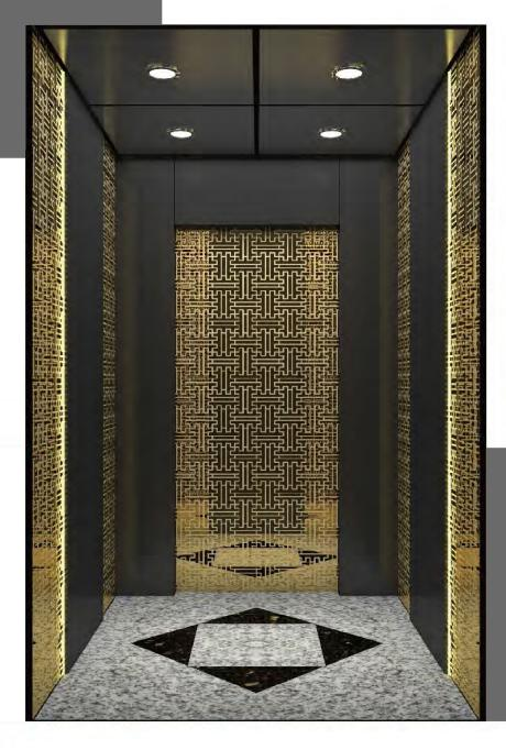
Ceiling: Ti-black mirror st.st. frame with downlight Car wall: Rear wall central panel Ti-gold mirror etched st.st., auxiliary panel Ti-black hairline st.st.; two side walls central panel Ti-black hairline st.st., auxiliary panel Ti-gold mirror etched st.st., soft light between central panel and auxiliary panel, Front wall Ti-gold mirror etched st.st.
